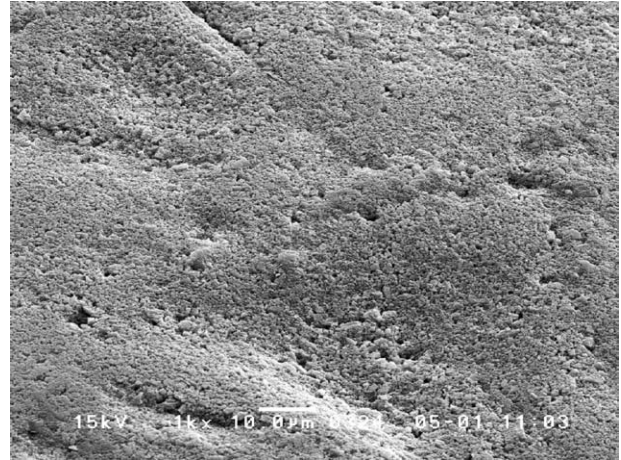
Figure 16 Scanning electron micrograph of paper coated with GCC based pigment (without thickener) and supercalendered at 87.5 kN/m and 50°C (Parker Print Surf. Roughness is 1.75 micron). Magnification = 1000×.
